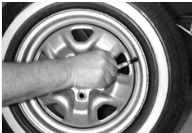
Figure 1 – Remove Valve Core to Deflate Tire
