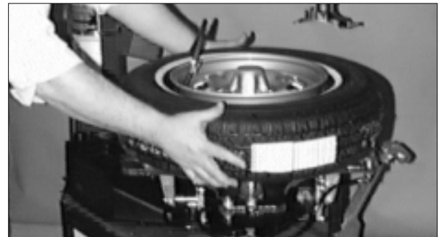
Figure 17 - Lift Tire Upwards for Bead Sealing
