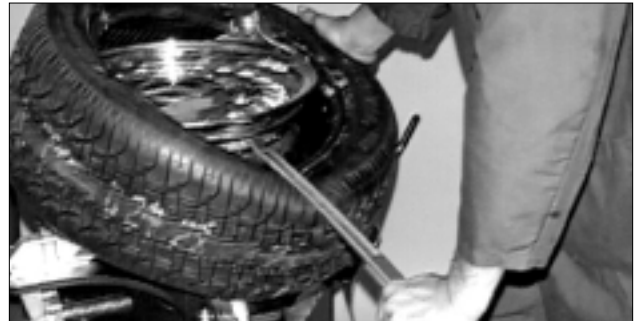
Figure 32 - Mount Upper Bead, Use Lifting Tool
