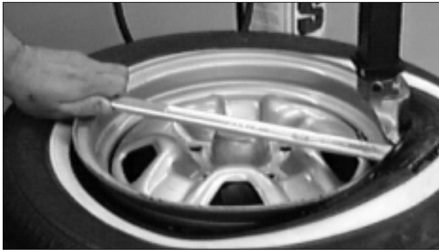
Figure 10 - Lift Bead Over Demount Head
