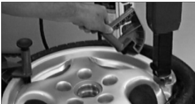
Figure 30 - Remove Drop Center Tools Before Tool Head
