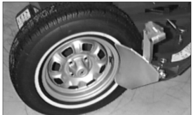
Figure 2 – Position Tire and Bead Loosener Shoe
