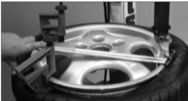
Figure 29 - Pull Lifting Tool Down and Rotate Wheel
