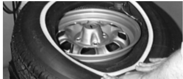
Figure 16 - Mounting Top Bead
