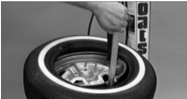
Figure 11 - Demounting Lower Bead
