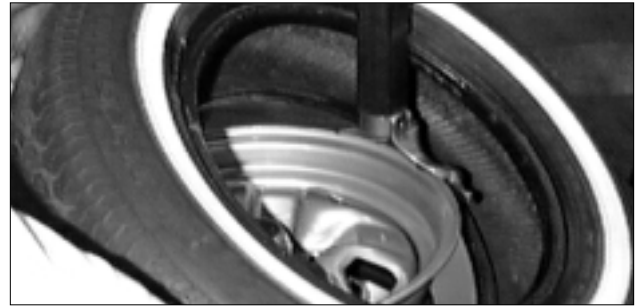
Figure 15 - Position Tire Against Mount/Demount Head
