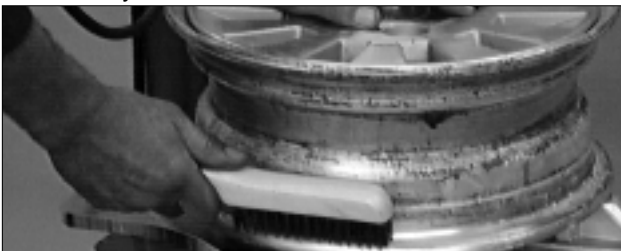
Figure 13 - Inspect and Clean the Wheel
