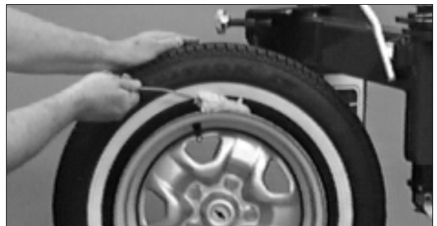
Figure 3 – Apply Rubber Lubricant to Tire Beads
