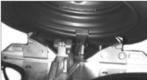
Figure 5 – Place Tire/Wheel Assembly on Table Top
