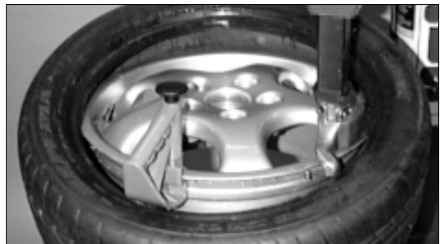
Figure 33 - Mounting Top Bead
